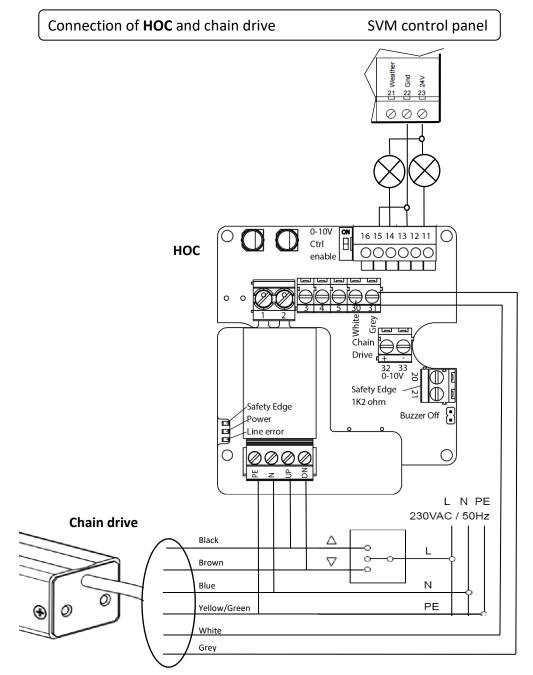
No further programming needed no matter chain length. Up to 4 chain drives in synchro.
