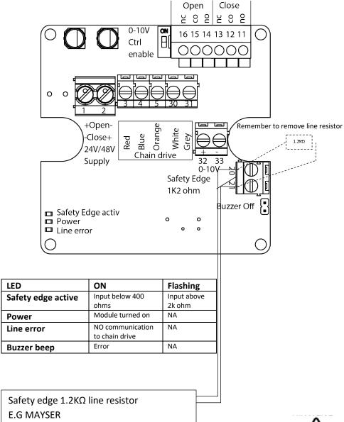
Remember to program Safety Edge Release distance in chain motor
