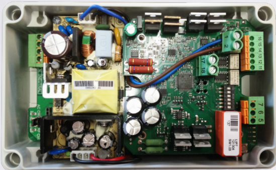
Flex1 ACDC as supply for built-in overload protector. ex. LIP7 OC #121308 Box size (LxWxH): 180 x 110 x 63 mm
